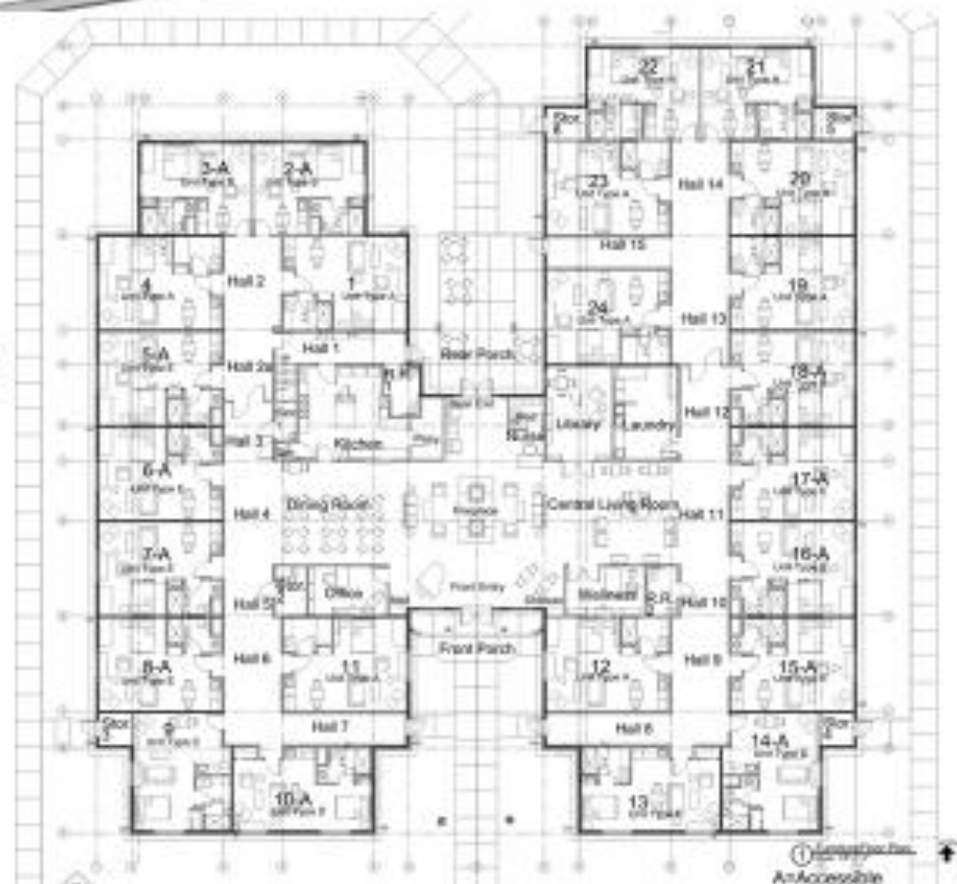
Assisted Living Facility – Prototype 17,000 s.f. 24 units - $2 milli
